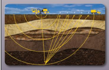
and models will help researchers understand the thickness and depth of the different types of underground rock layers. This information is critical for assessing, conducting and monitoring a carbon storage project.
